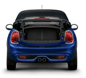
The soft top of the MINI Cabrio opens electrically in 20 seconds – even with the car moving at up to 30 km/h. When the top is closed the multiple layers of fabric make for excellent sound insulation and comfort on long journeys.
