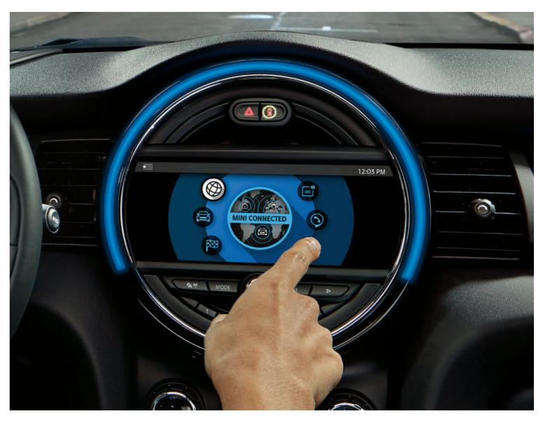
Harking back to the classic Mini with the round speedo in the middle of the dashboard: the MINI Centre Instrument. 16.4 cm/ 6.5" display screen and Bluetooth telephony are standard features and there are three enhancement levels – from the
